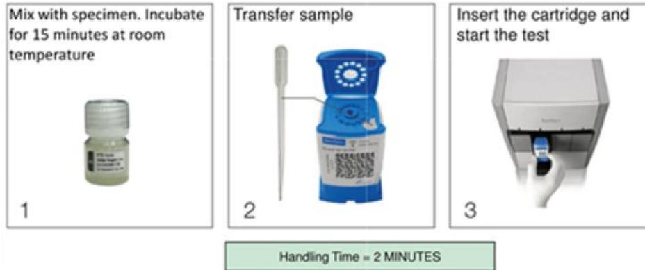
Once cartridge is ready, test should be loaded within 30 minutes.
